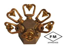
Proprietary and unique to both the ACAF® Deluge and Fixed Spray Systems is the DN 7 Nozzle. Patent and FM Ap- proved for installation in the pendant and horizontal positions, these multi-port nozzles are highly cost effective as they allow for the greatest spacing possible, to minimize the amount of nozzles and piping needed.
